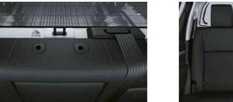
**CRS top tether anchor:** Enables the fixing of an ISOFIX-compliant child seat on the outboard rear seats.
